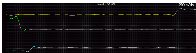
Figure 4-20: the U_s (yellow), U_c (green) signals and the estimated angle (blue) for a step change from 50 to 80 degrees.
