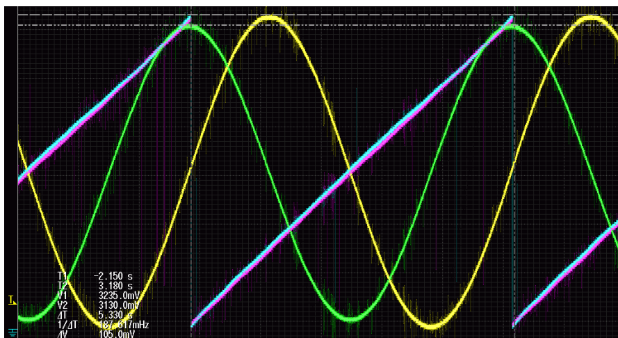
Figure 3-14: The U_S and U_C signals (yellow and green respectively), the estimated angle before correction (blue) and the estimated angle after correction signal (pink) for case 2.
